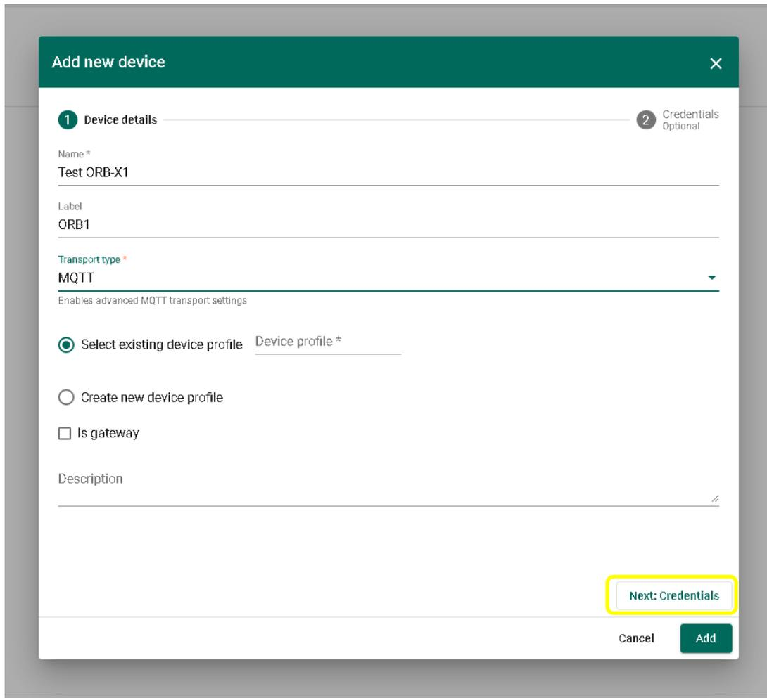
Figure 3 - Device Detail
